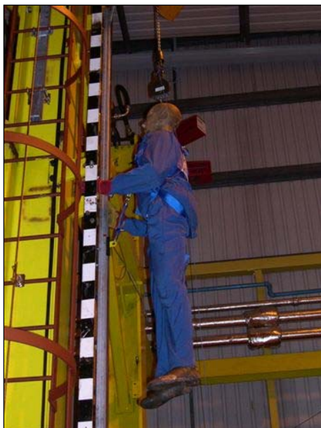
FIGURE 7 TEST 4: FALL DOWN TEST PRE- DROP FALL POSITION
