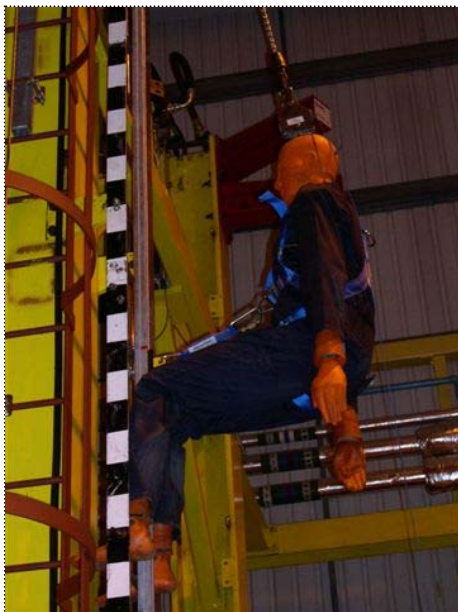
FIGURE 11 TEST 6: SIT BACK TEST PRE- DROP FALL POSITION
