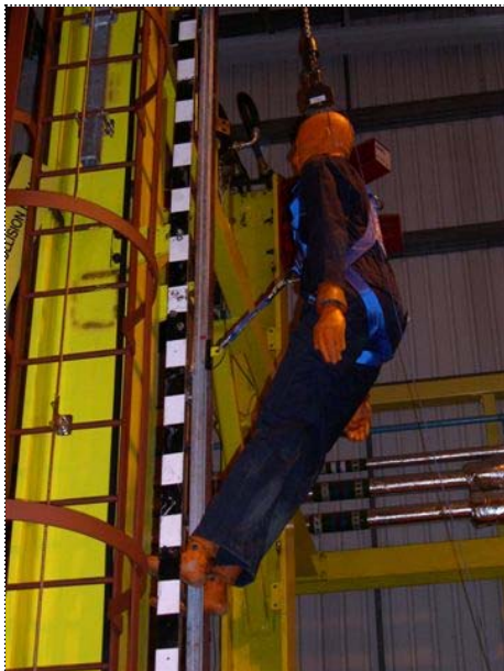
FIGURE 9 TEST 5: FALL BACK TEST PRE- DROP FALL POSITION
