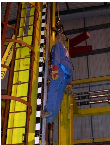
FIGURE 1 TEST 1: FALL-BACK TEST PRE- DROP FALL POSITION
