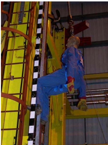
FIGURE 3 TEST 2: SIT-BACK TEST PRE- DROP FALL POSITION
