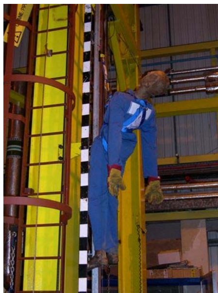
FIGURE 2 TEST 1: FALL-BACK TEST POST- DROP REST POSITION
