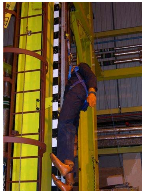
FIGURE 14 TEST 7: CLIMB-FALL TEST POST- DROP REST POSITION
