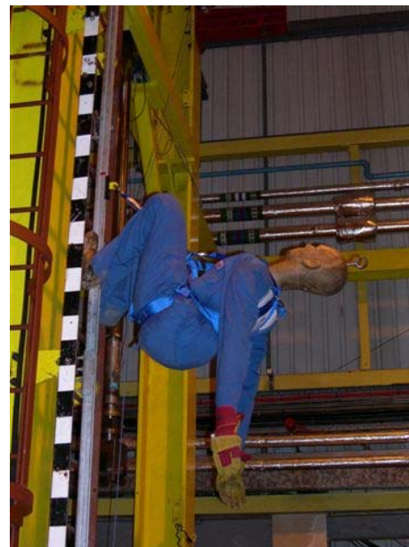
FIGURE 4 TEST 2: SIT-BACK TEST POST- DROP REST POSITION
