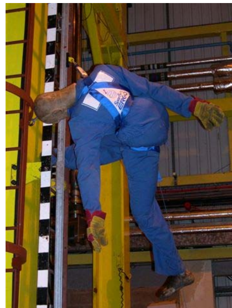
FIGURE 6 TEST 3: CLIMB-FALL TEST POST- DROP REST POSITION
