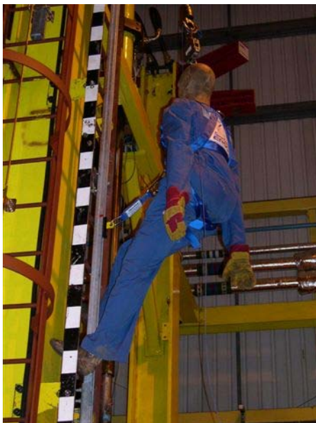
FIGURE 5 TEST 3: CLIMB-FALL TEST PRE- DROP FALL POSITION
