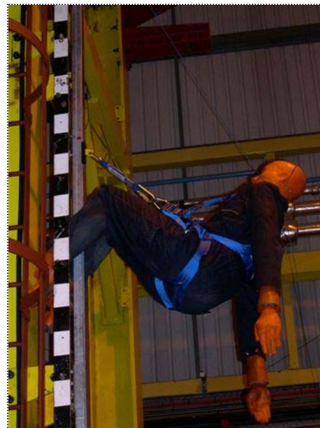
FIGURE 12 TEST 6: SIT BACK TEST POST- DROP REST POSITION
