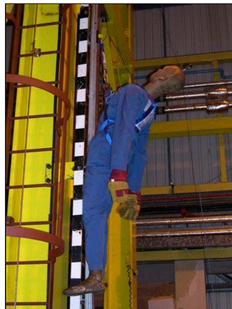
FIGURE 8 TEST 4: FALL DOWN TEST POST- DROP REST POSITION
