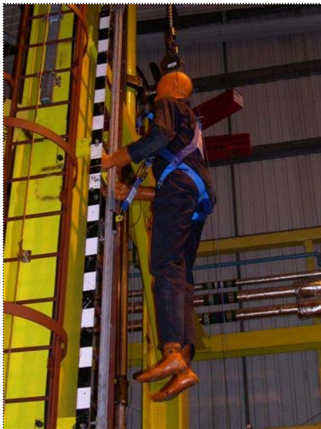
FIGURE 15 TEST 8: FALL DOWN TEST PRE- DROP FALL POSITION
