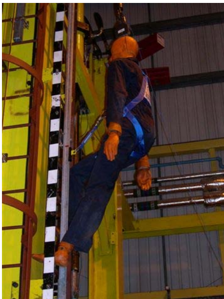
FIGURE 13 TEST 7: CLIMB-FALL TEST PRE- DROP FALL POSITION
