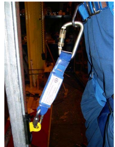
FIGURE 3 GUIDED FALL ARRESTER MOUNTED ON RAIL
