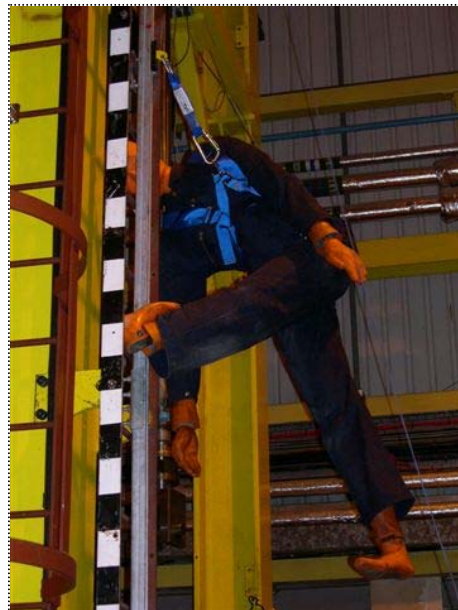
FIGURE 10 TEST 5: FALL BACK TEST POST- DROP REST POSITION
