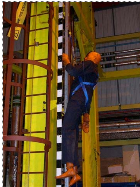
FIGURE 16 TEST 8: FALL DOWN TEST POST- DROP REST POSITION
